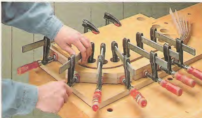
3 Now clamp the corner pressure block against the strips. If the strips slide up, simply tap them back down against the base, see tip in margin.
