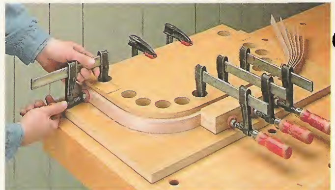
2 Before adding the next pressure block, bend the strips the rest of the way around the form and “corral” the ends by positioning a clamp loosely around them.
