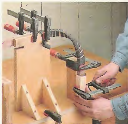
5 To ensure the edges of the strips bottom out against the stop, clamp the alignment block in place.
