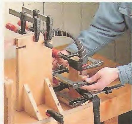
6 Squeeze the strips tight against the support block by applying clamping pressure in the other direction.
