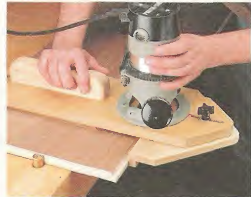
Edge Guide. By replacing the stop with a triangular-shaped edge guide, you can rout rabbets quickly and accurately with an ordinary straight bit.
