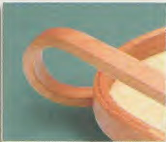
B. Compound Curve. To create a compound curve, the wood strips are bent and twisted around a jig to form a dramatic bent wood shape.
