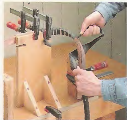
3 To anchor the tubing, clamp it to the upright. Then stretch the tubing tight as you wrap it around the bend.
