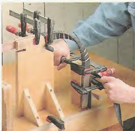
4 When you've wrapped the tubing all the way around the bend, clamp it tightly against the support block.
