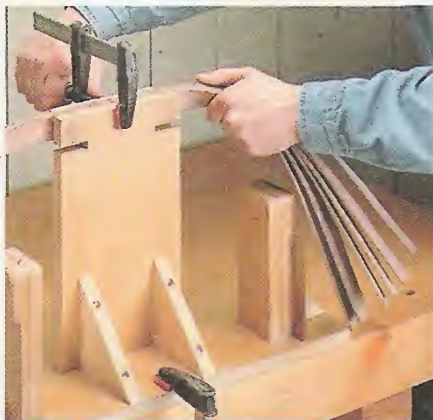
1 Start by centering the strips on the upright and clamping them in place so the edges align with the top.
