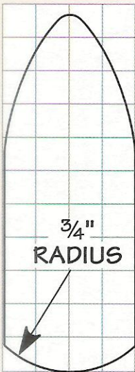
▲ Use this full-size pattern to make a template of the curved ends of the plates as well as the torpedo shape of the level.
