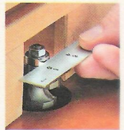
▲ With a metal rule held on edge, it's easy to align the fence so it's flush with the bearing.
