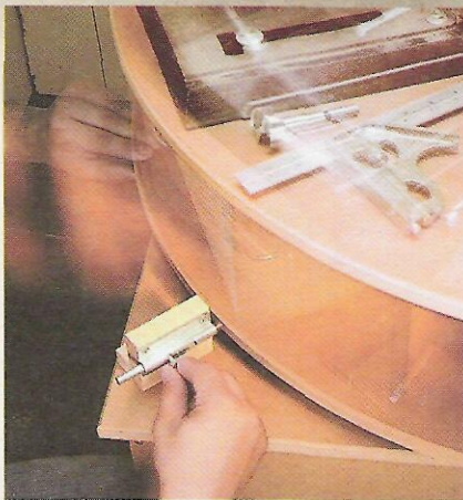
A. Carousel. Just spin the carousel to put the tool you need directly in front of you. Then lock it in place.
