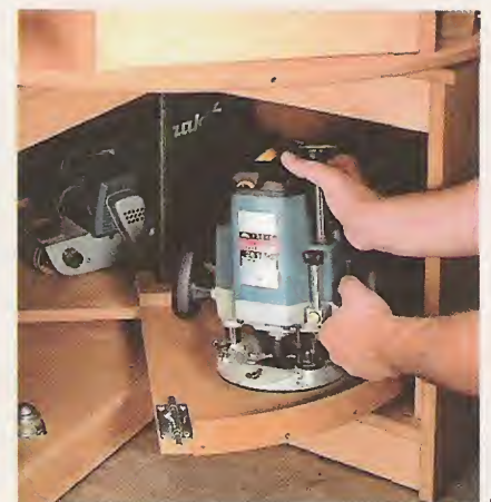
C. Turntable. A spin of the turntable in the base provides quick and easy access to portable power tools.
