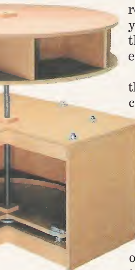
To provide easy access to your benchtop tools, the carousel spins on the roller bearings attached to the top of the base.
