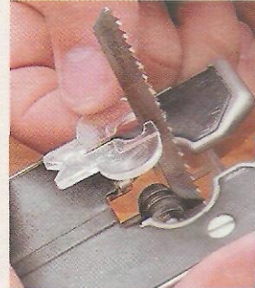
To prevent chipout, all the sabre saws except the Porter Cable have a plastic insert that fits in the base.
