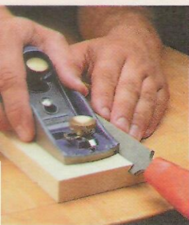
Setting a file in a scrap with a 45° saw kerf makes it easy to create a uniform chamfer on the bottom edges of the plane.
