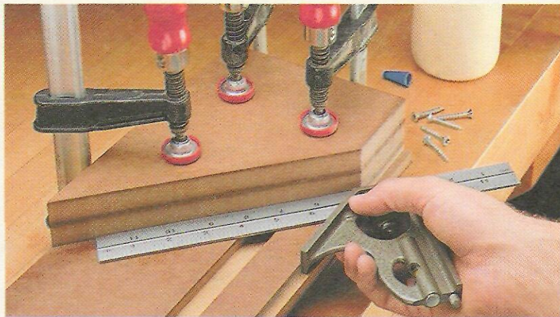
▲ The accuracy of the miter trimmer is "built in" by carefully positioning the angled platform. Using a combination square, set it at a 45° angle to the track for the block plane. Then glue and screw it to one side only.
