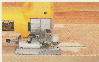
▲ Dust Control. A blower in each saw directs dust away from the blade so you can see the layout line as you make a cut (left). In addition, the Bosch (right) and Milwaukee each have a port for hooking up a shop vacuum.
