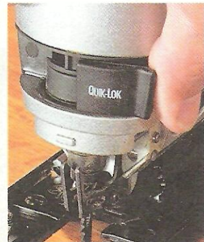
▲ Blade Changing. While the Hitachi (left) requires a wrench to change blades, the DeWalt (center) only takes a couple turns of a knob. Even so, it's not as quick as the spring-loaded lever on the Milwaukee (right).
