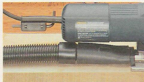
▲ Dust Control. A blower in each saw directs dust away from the blade so you can see the layout line as you make a cut (left). In addition, the Bosch (right) and Milwaukee each have a port for hooking up a shop vacuum.
