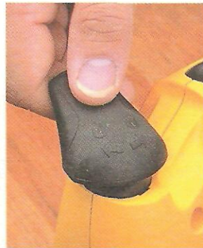
▲ Blade Changing. While the Hitachi (left) requires a wrench to change blades, the DeWalt (center) only takes a couple turns of a knob. Even so, it's not as quick as the spring-loaded lever on the Milwaukee (right).
