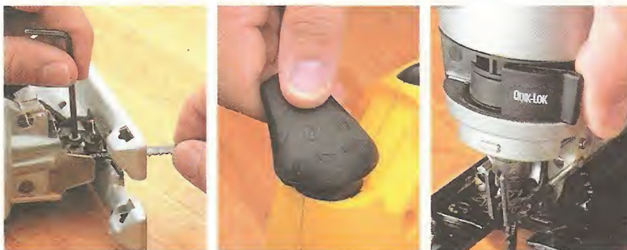
▲ Blade Changing. While the Hitachi (left) requires a wrench to change blades, the DeWalt (center) only takes a couple turns of a knob. Even so, it's not as quick as the spring-loaded lever on the Milwaukee (right).
