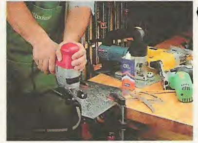
Test Procedures. A sabre saw has an incredibly tough job — making a controlled, accurate cut in all different kinds of materials. To test the performance of these saws, we plowed through 2"-thick oak (left), made intricate scroll cuts in plywood (center), and sawed heavy-gauge metal (right).
