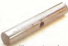
It's easy to make the cross-dowel. After cutting a short length of steel rod, drill a \frac{13}{64} "-dia. hole and cut the threads with a \frac{1}{4} -20 tap.
