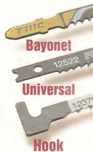
Most sabre saws accept bayonet (top) or universal blades (middle). The hook blade (bottom) only fits the Porter Cable.
