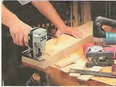
Test Procedures. A sabre saw has an incredibly tough job — making a controlled, accurate cut in all different kinds of materials. To test the performance of these saws, we plowed through 2"-thick oak (left), made intricate scroll cuts in plywood (center), and sawed heavy-gauge metal (right).
