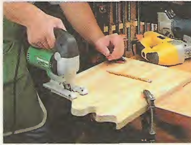
Test Procedures. A sabre saw has an incredibly tough job — making a controlled, accurate cut in all different kinds of materials. To test the performance of these saws, we plowed through 2"-thick oak (left), made intricate scroll cuts in plywood (center), and sawed heavy-gauge metal (right).
