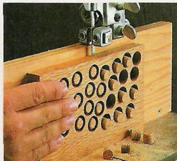
2 Now clamp a tall auxiliary fence to the bandsaw table and cut the plugs free.
