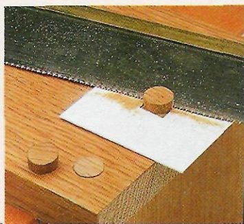
5 Set posterboard over the plug to protect the workpiece as you saw off the waste.
