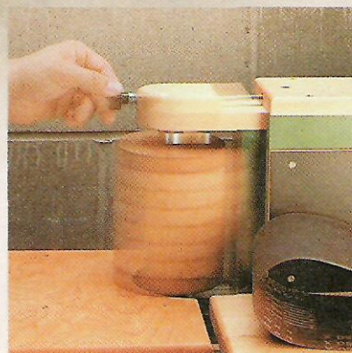
▲ Changing Belts. A quick-release tension device makes it easy to change sanding belts.
