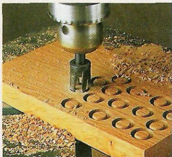
1 With a plug cutter chucked in a drill press, cut the plugs in a scrap from the project.
