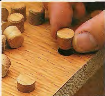
3 Select a plug for each hole that matches the grain and color of the surrounding wood.
