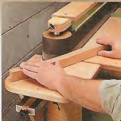
▲ Curved Pieces. An end table "wraps" around a roller so you can sand curved workpieces.
