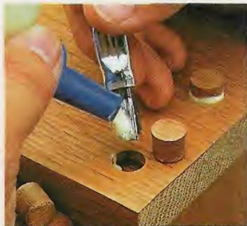
4 After brushing glue around the sides of the hole, tap the plug in place so it's snug.
