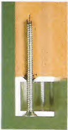
▲ A countersink on the bottom of the aluminum channel recesses the screw head. The one on top forms a pocket for any wood fibers that pull out as you drive in the screw.
