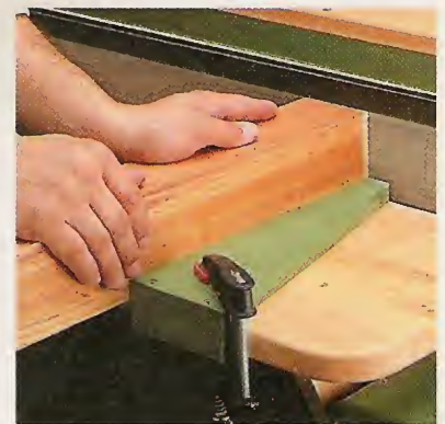
▲ Stop. Clamping a stop to the front table allows you to sand the ends of a workpiece square.
