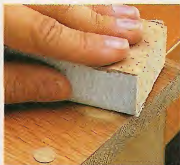
6 Finally, sand each of the plugs flush with the surface of the workpiece.
