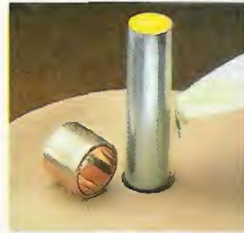
▲ A slow-setting epoxy fills the gap between the shaft and the drive roller. Before it "welds" them together press a bushing into the opening.
