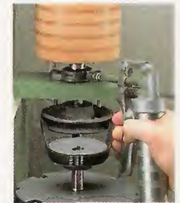
▲ Be sure to keep the flange bearings greased to prevent them from overheating.
