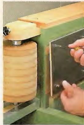
▲ To make the platen easy to replace if it gets worn, it's simply screwed to the sleeve.
