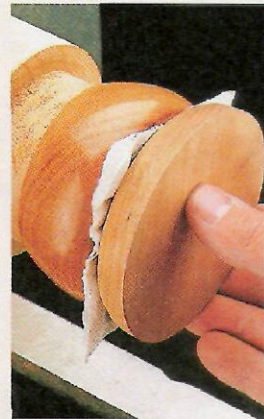
A paper towel slipped between the lid and box will help tighten up a loose-fitting lid so you can turn both to final shape.
