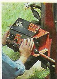
8 As the blade slices through the log (left), the feed rate is controlled by the sawyer (center). A gauge (right) helps determine the thickness of the board.
