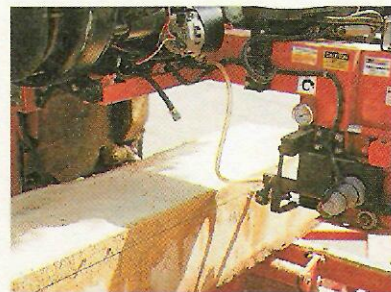
10 To prevent pitch from gumming up the blade, a water-drip system keeps it running cool.
