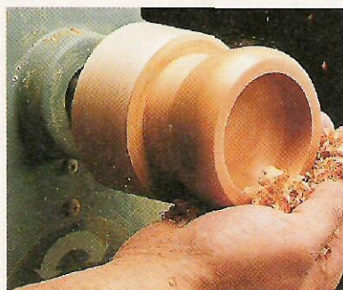
B. Burnishing. To produce a nice sheen, hold a handful of shavings against the workpiece as it turns.
