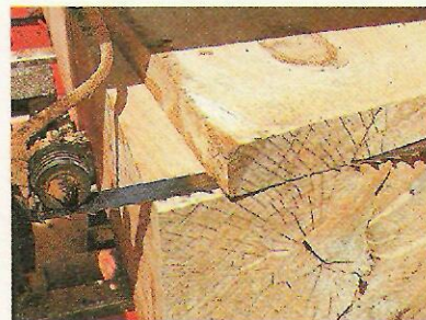
11 A sharp blade and a mill that's properly aligned will produce quality boards like this.
