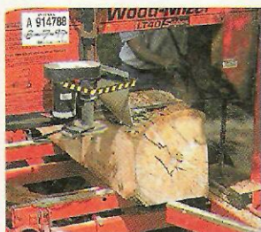
7 During the initial cut, the blade removes the top portion of the log (left). Then the log is rotated to square up the remaining sides (right).
