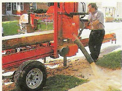
9 Dust pours out a chute on the side of the mill as the head of the saw travels along a steel rail.
