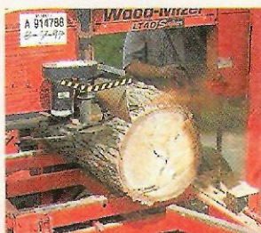
7 During the initial cut, the blade removes the top portion of the log (left). Then the log is rotated to square up the remaining sides (right).
