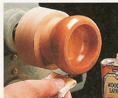
C. Finishing. After applying a finish, use a cloth to distribute it evenly as the workpiece turns.
