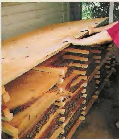
5 Adding a final piece of plywood keeps the top layer of lumber from drying too quickly.
