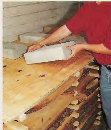
6 The stack is weighted down with concrete blocks to prevent the top boards from warping.
