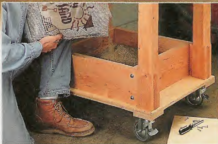
A. Sandbox. To add stability, a “sandbox” in the bottom of the stand holds about 100 lbs. of sand. This extra ballast prevents the stand from tipping when you roll it around.
