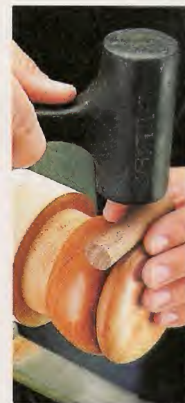
To remove a tight fitting lid, gently tap a dowel along the joint line between the lid and box.
