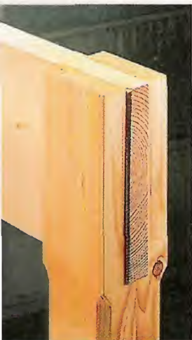
▲ A strong mortise and through tenon joint provides the cornerstone for a sturdy base.
