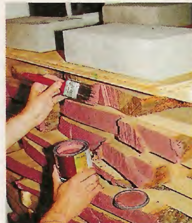
7 To minimize checking caused by losing moisture too rapidly, paint the ends of the boards.
