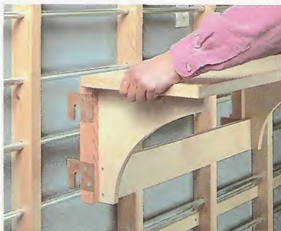
▲ It's easy to hang each storage unit exactly where you want on the grid (left). The secret is a set of hanging brackets attached to the back of each unit that fit securely over the metal conduit (right).
