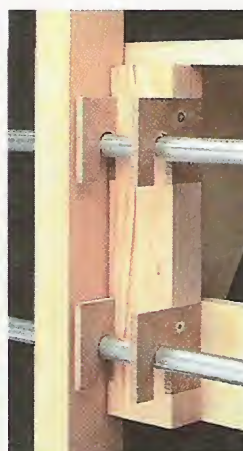
▲ It's easy to hang each storage unit exactly where you want on the grid (left). The secret is a set of hanging brackets attached to the back of each unit that fit securely over the metal conduit (right).
