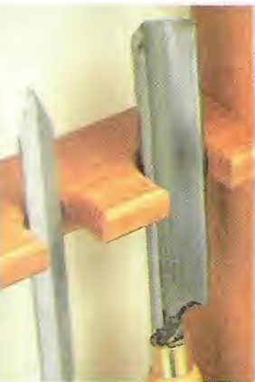
▲ To hold the large blade of my roughing gouge, I cut one notch a bit wider and deeper than the others.
