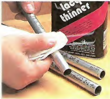
▲ All it takes to "erase" the black print on the conduit is to wipe it off with lacquer thinner.
