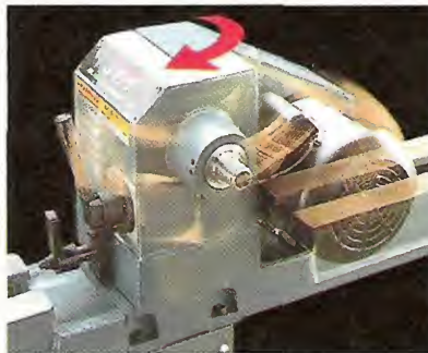
▲ Outboard Turning. The headstocks on all these lathes can be rotated 90° to the bed (left). This lets you turn large diameter workpieces. And it positions the workpiece for easy access (right).
