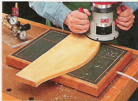
◀ Vacuum Table. To hold a workpiece securely in place, a vacuum is formed on the surface of this compact table.
