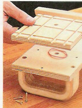
▲ Slipping an ordinary rubber band between the base of the routing jig and the vacuum plate creates an airtight seal.
