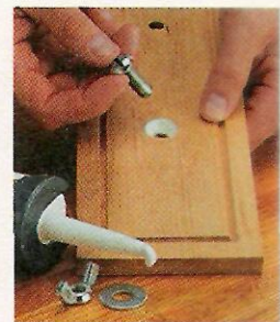
▲ To seal the hole in the base of the featherboard, squeeze caulk in the counterbore before installing the bolt.
