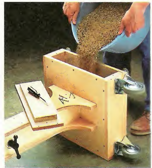
▲ Sand. To provide extra ballast that keeps the support stand from tipping, remove one side of the base and fill it with sand.
