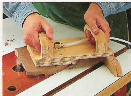
▲ Routing Jig. A vacuum allows this jig to hold small parts so you can rout them safely on a router table.
