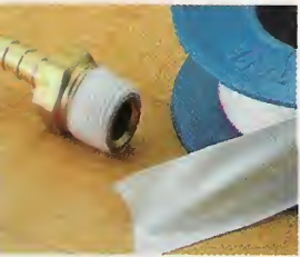
▲ To produce an air-tight seal, wrap the threads of the brass fitting with Teflon tape before screwing it in place.
