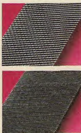
The diamond-shaped cutting edges on a double-cut file (top) remove material more aggressively than a single-cut file (bottom).
