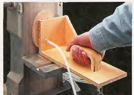
▶ Small-Piece Sanding Jig. A vacuum plate in the front of this jig makes it easy to sand small workpieces safely.
