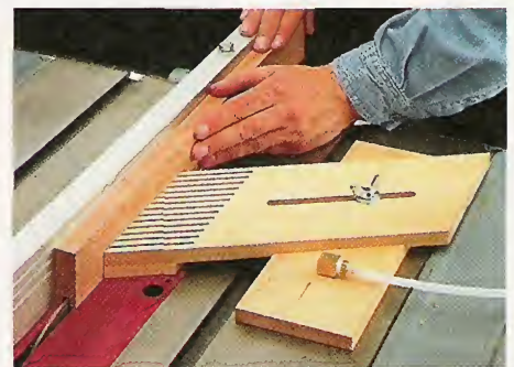
▲ Featherboard. All it takes to attach this featherboard to a table saw is to flip a switch on the vacuum system.
