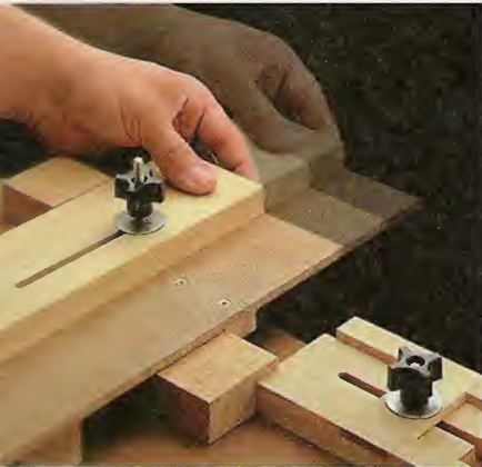
▲ To reduce chipout, just slide the fence in so a small backup block butts up against the workpiece.
