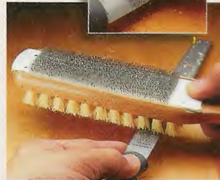
File Card. Nylon bristles on this file card brush off the loose dust. And steel wires remove material that gets packed in, see inset.
