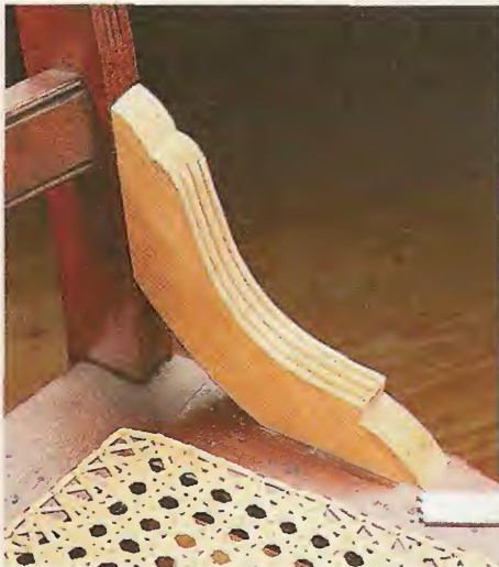
Repair. To repair a piece of furniture, just file a cutter to produce a detail that matches the one on the damaged part.
