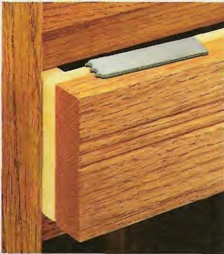
Beads. The beads on this drawer front were shaped with a single cutter — yet they can't be duplicated with a router bit.
