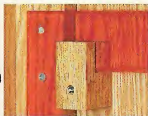
◀ To hold the T-square, the blade is supported at each end by a thick block of hardwood with a kerf in it.
