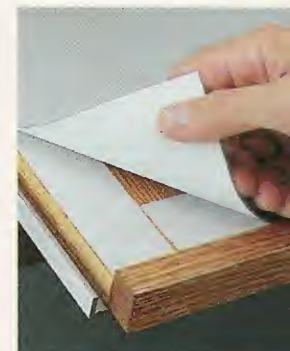
▲ Strips of carpet tape are all that's needed to attach the Borco cover to the table.
