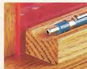
A scooped out block acts as a pencil tray. Setting the block in from the back lets you slip triangles behind it.
