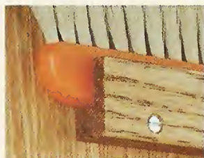
▲ The plastic back of a brush rests in a rabbeted block that's screwed to the back of the case.
