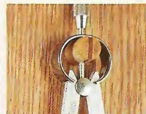
▲ An ordinary dowel with a kerf cut in one end provides a simple hanger for a compass.
