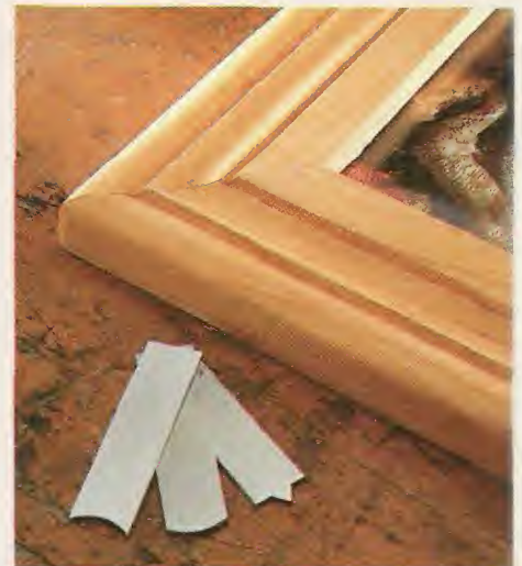
Multiples. By using several cutters, you can produce a complex molding like the one on this picture frame.
