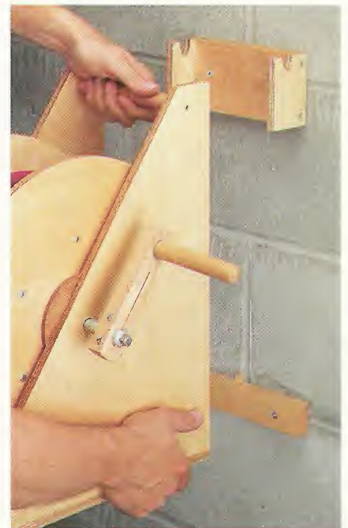
Portable. Two simple brackets let you hang the hose reel on the wall or remove it to use away from the shop.
