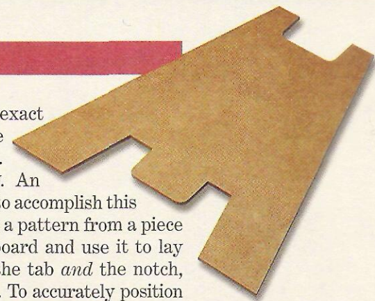
▲ A hardboard template provides a quick way to make identical end pieces.
