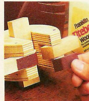
▲ To produce a no-slip surface, I glued strips of cloth-backed sandpaper (100-grit) to the ends of the curved fingers.
