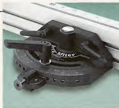
Head Styles. The Accu-Miter (left), Vega, and Inca have a traditional protractor-style head. But the Osborne uses a telescoping arm that connects the fence and miter bar to create a stable, triangular "head."
