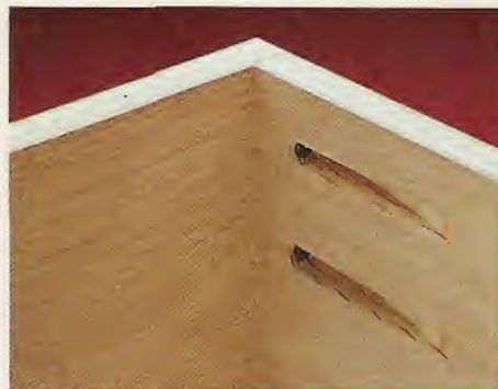
Cabinets. The jig also makes it easy to cut the pockets and drill the pilot holes that are used to assemble this cabinet.
