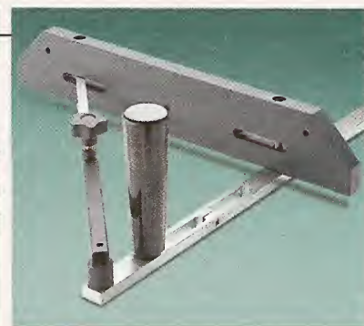
Head Styles. The Accu-Miter (left), Vega, and Inca have a traditional protractor-style head. But the Osborne uses a telescoping arm that connects the fence and miter bar to create a stable, triangular "head."
