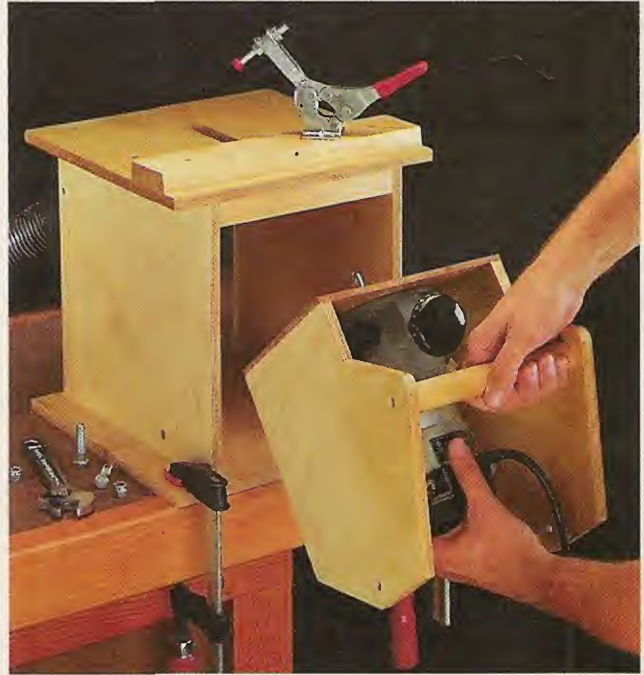
▲ Pocket Hole Jig. Setting up our Pocket Hole Jig (shown on page 16) is easy. That's because the router that cuts the pocket is mounted in a removable carriage.
