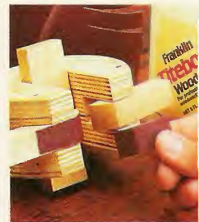
▲ To produce a no-slip surface, I glued strips of cloth-backed sandpaper (100-grit) to the ends of the curved fingers.
