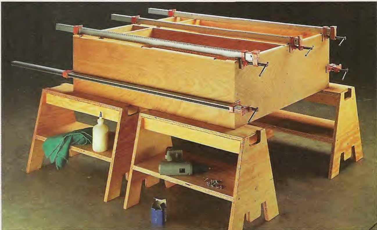
▲ Stacking Sawhorses. Building a large project? This set of four Stacking Sawhorses provides a handy assembly area. Unlike a workbench that's often
