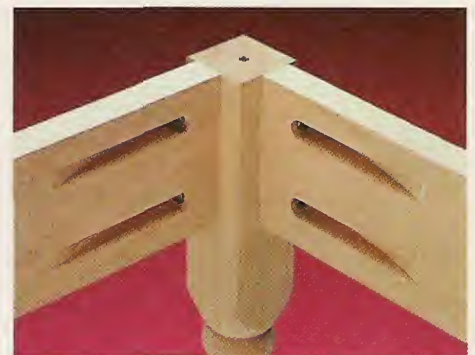
Furniture. After using the jig to cut the pockets in the base of this table, installing screws provides plenty of strength.
