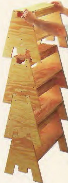
▲ When it's time to "stable" your sawhorses, they don't take up much floor space. Just stack all four together for storage.
