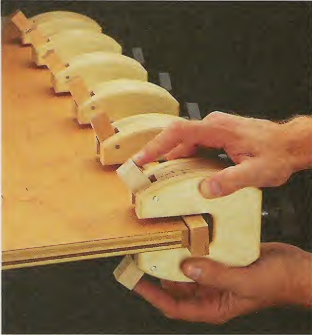
▲ Edge Clamps. To release these Edge Clamps from the workpiece, simply loosen the lock knob and push the spring-loaded "fingers" forward. (Plans begin on page 6.)
