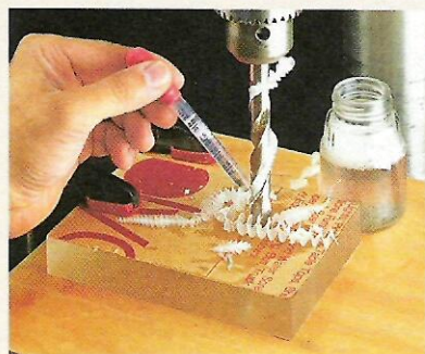
D. Lubricant. Soapy water acts as a lubricant that allows the drill bit to cut thin, feathery shavings.
