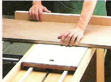
B. Slick. This cutoff table rides on pieces of plastic laminate, so it slides smoothly without binding.
