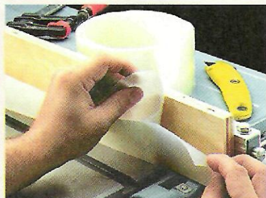
F. Fences. To make a workpiece slide easily along an auxiliary fence, add a strip of UHMW plastic.
