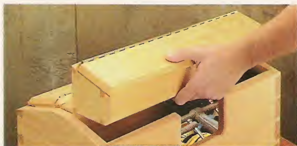
B. Notch. A large notch lets you lift out the bins to remove the tools stored below. For small jobs that only require a few items, just take the bin with you.
