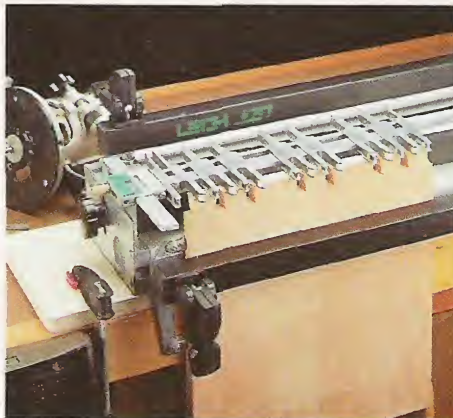
Leigh Dovetail Jig. It's hard to beat the versatility of this jig. The unique design of the fingers lets you rout through-dovetails, half-blind dovetails, and even sliding dovetail joints.
