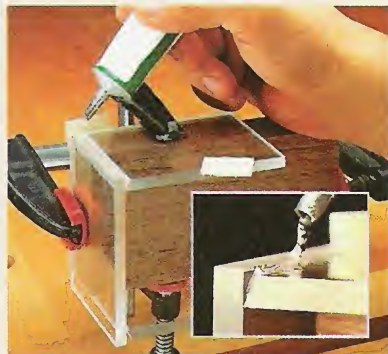
G. Polymerized Cement. For a strong joint, bevel one piece before applying polymerized cement.
