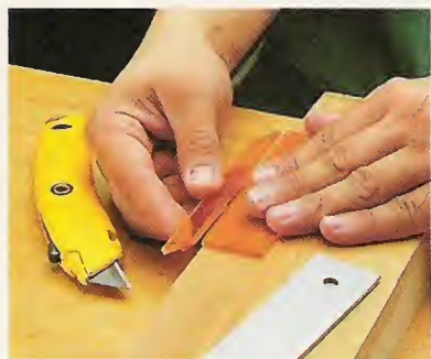
A. Score & Snap. To cut thin pieces of plastic, simply score a line and snap it over a scrap.
