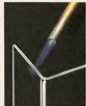
To polish the rough edge on acrylic or polycarbonate, sweep the flame from a torch slowly across the surface.
