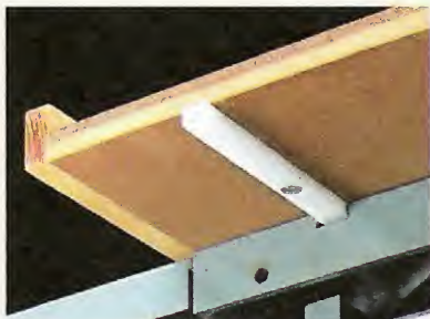
E. Runners. Jigs slide easily when they're guided by a runner made from a piece of UHMW plastic.
