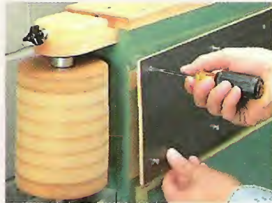
A. Durability. Plastic laminate creates a tough, durable surface on the platen of this edge sander.
