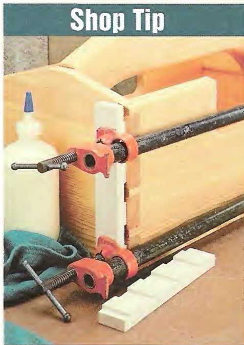
▲ The notches in these blocks form pads that allow you to apply clamping pressure directly against the tails.
