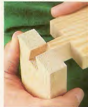
▲ To produce a "near fit," the pin should almost (but not quite) fit into the opening between the tails.
