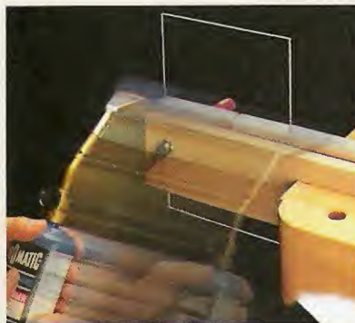
H. Propane Torch. After sandwiching the plastic between a scrap and a bending form, heat along the bend line (left). Once the plastic has softened, bend it over the form and allow it to cool (right).
