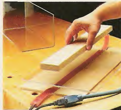
I. Strip Heater. A strip heater makes it easy to create a uniform bend in a long piece of plastic.
