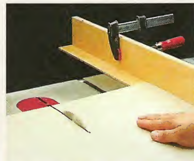
C. Table Saw. An L-shaped fence keeps the plastic laminate from slipping under the rip fence.
