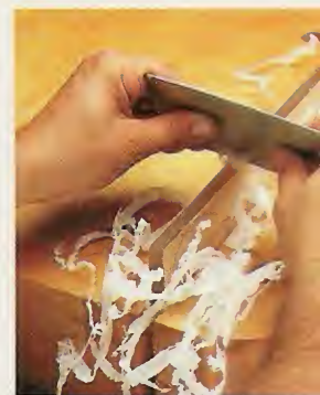
An ordinary hand scraper makes quick work of removing saw marks from a piece of plastic.
