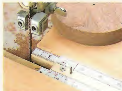
H. Indicator. A hairline mark on a piece of acrylic makes it easy to precisely set a measurement.
