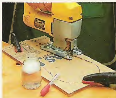
B. Sabre Saw. When making a cut with a sabre saw, soapy water prevents the plastic from melting.
