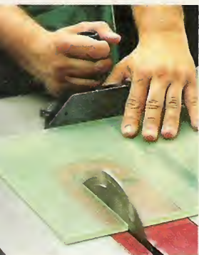
Raising the saw blade about 1" above the plastic reduces the amount of heat that builds up and produces a smooth, clean cut.
