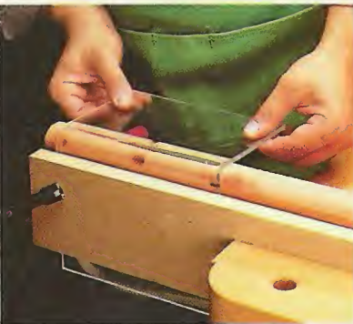
H. Propane Torch. After sandwiching the plastic between a scrap and a bending form, heat along the bend line (left). Once the plastic has softened, bend it over the form and allow it to cool (right).
