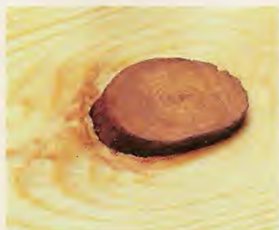
A. Loose Knots. A black ring around a knot is a sign that a knot will loosen up over time.
