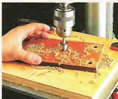
E. Chamfer. Before cutting threads in plastic, chamfer the rim of a hole to ensure a flat, level surface.
