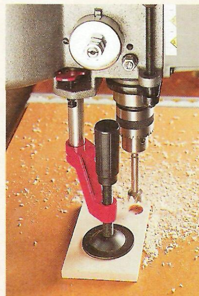
C. Hold-Down. The hold-down is a good idea. But since it won't tighten down, it's nearly useless.
