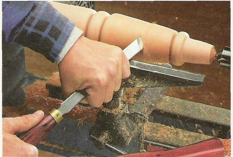
▲ From planing a smooth finish to turning a bead, a skew chisel is a versatile turning tool.
