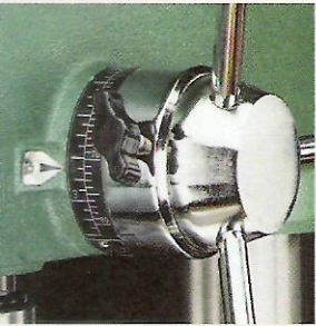
▲ A locking collar on the Grizzly and Bridgewood lets you quickly “dial in” the depth of hole.
