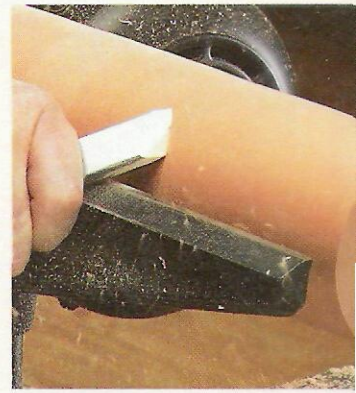
▲ A planing cut (and a light touch) will produce a smooth surface that doesn’t need sanding.
