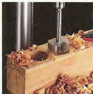
C. Power. To see if the drill presses would bog down in a heavy cut, we bored a series of large, deep holes.
