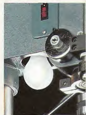
▲ A 60-watt light in the head of each drill press makes it easy to see when positioning work under the bit.
