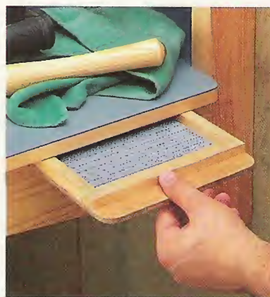
B. Sliding Tray. A tray slides out of either side of the station to hold the tools you're working on.
