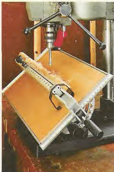
B. Tilting Table. A tilting table and fence make it easy to support long workpieces and drill angled holes.
