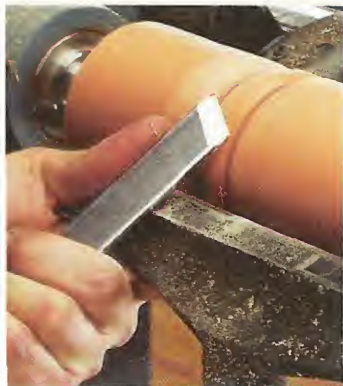
▲ The secret to turning the curved shoulders of a bead is to roll the skew chisel in one continuous motion.
