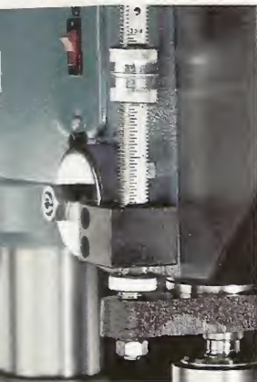
▲ But tightening two nuts on a threaded post creates a more reliable depth stop on the Jet and Powermatic .
