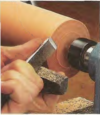
▲ Peeling off a sliver of wood with a facing cut makes it easy to square up the end of a spindle.
