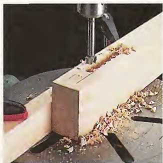
B. Performance. By drilling dozens of mortises with each drill press, we got a feel for overall performance.
