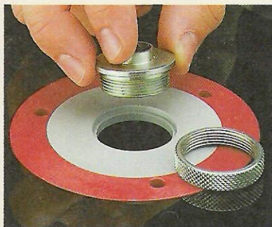
▲ Guide Bushing. If you do a lot of template routing, it's handy if the insert accepts a guide bushing.
