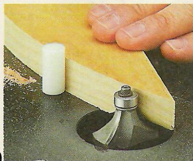
▲ Starting Pin. Using a starting pin prevents the bit from grabbing the workpiece at the beginning of a cut.
