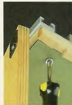
▲ An adjustment screw lets you "tweak" the wings to create a flat, level worksurface.
