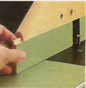
▲ To quickly adjust the fence opening for different size bits, just move the sliding faces in or out as needed.
