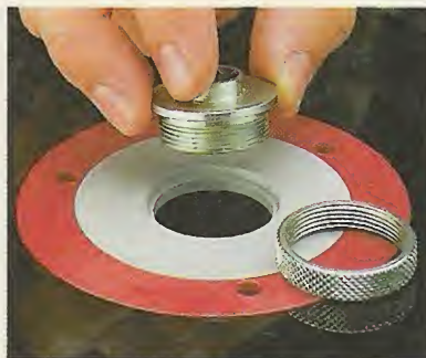
▲ Guide Bushing. If you do a lot of template routing, it's handy if the insert accepts a guide bushing.
