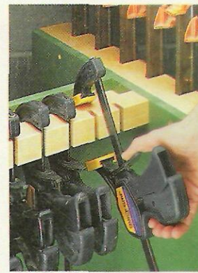
▲ To hold this quick clamp in place, the curved jaw hooks over a lip on the hanger.
