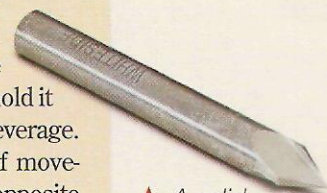
▲ A solid carbide V-groove bit used to cut the threads won't need sharpening nearly as often as the cutter in the threadbox.
