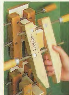
▲ All it takes to hold handscrews is a simple wood block.
