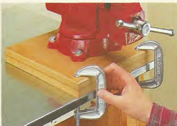
▲ Mounting Pads. A double layer of MDF provides a solid mounting pad for a vise (or grinder). Clamping the pad to the metal cover holds the tool securely in place.
