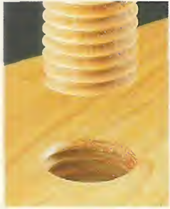
To adjust the height of the seat, the post threads into the hole in the lower support.
