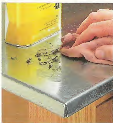
A. Metal Cover. The metal cover on the workbench cleans up easily. And solvents won't damage the surface.
