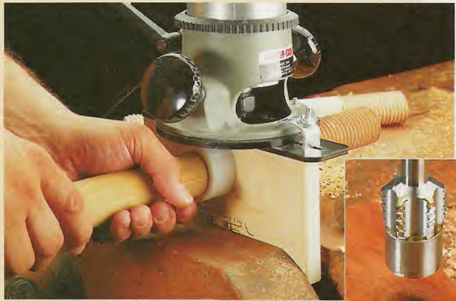
▲ To rout the outside threads in a dowel, twist it through the plastic insert in this jig like you're making sausage. A hand-held tap cuts the inside threads, see inset photo.
