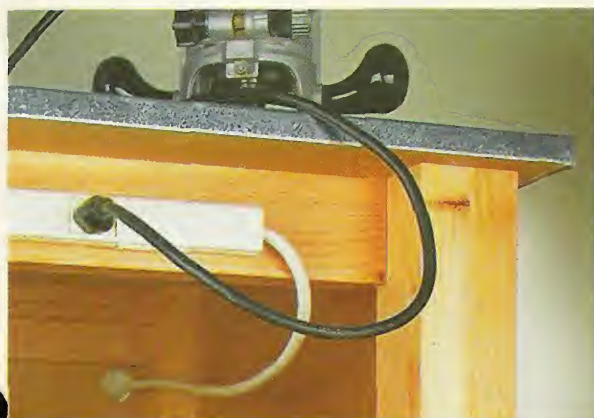
▲ Power Strip. To provide a convenient plug-in for my portable tools, I attached a power strip to the bench. The power cord for the strip feeds out a hole in back.
