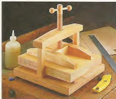
▲ Veneer Press. Tightening a single wood screw applies all the clamping pressure that's needed for this small veneer press.
