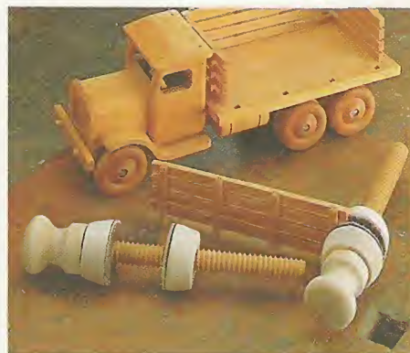
▲ Small-Piece Clamps. These clamps are ideal for delicate work. Just thread a short dowel. Then tap threads in the lower nut.
