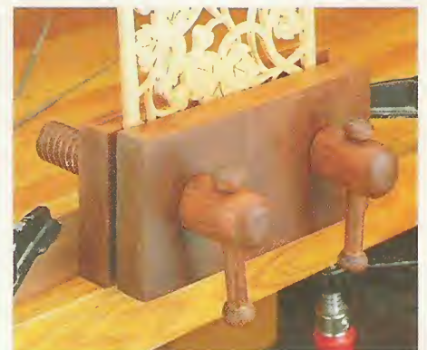
▲ Benchtop Vise. The twin wood screws on this small, benchtop vise thread into tapped holes in the back jaw.
