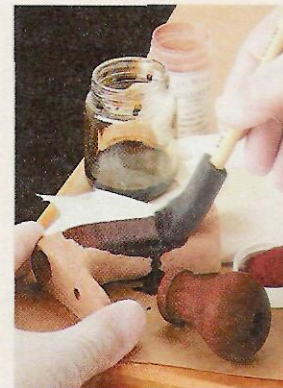
▲ Brushing on an aniline dye (Cuban red mahogany) creates a traditional dark-colored handle.
