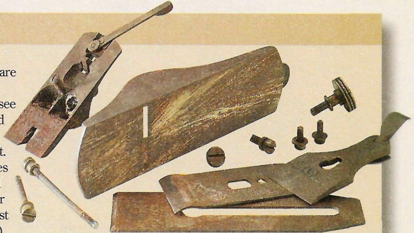
▲ Heavy pitting on the back side of the blade made it impossible to get a sharp cutting edge.
