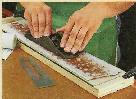
A. Sandpaper. To remove rust from the sole, I "scrubbed" the plane across sandpaper attached to a piece of glass.
