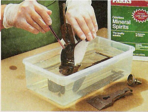
▲ Mineral Spirits Bath. To loosen rust and grime, soak the metal parts of the plane in mineral spirits. Then scrub each part clean with a brush and set it aside to dry.
