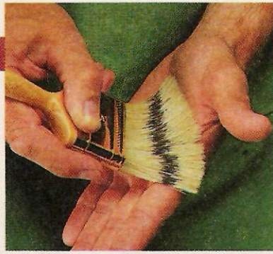
A. Remove Dust & Bristles. Work the brush back and forth in your palm to remove dust or loose bristles.
