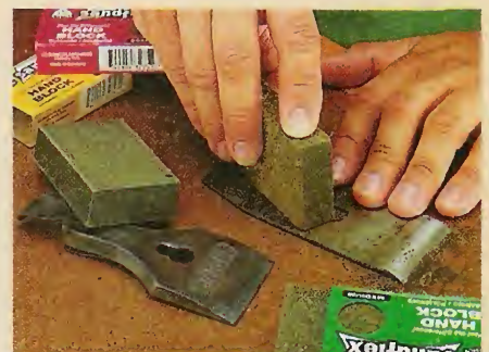
C. Eraser Blocks. These rubber blocks embedded with silicon carbide work great for "erasing" rust from metal parts.
