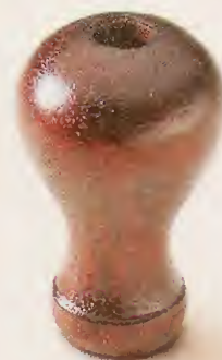
▲ Making a new front knob to replace a damaged one is easy. Just turn a scrap block to shape on the lathe.
