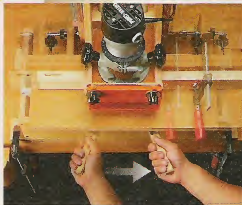
B. Length. To cut the mortise to length, use the handle to slide the table from side to side. Two stops control the amount of movement.
