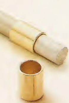
▲ Bronze bushings that slip over the metal guide rods create an accurate guide system for the carriage.
