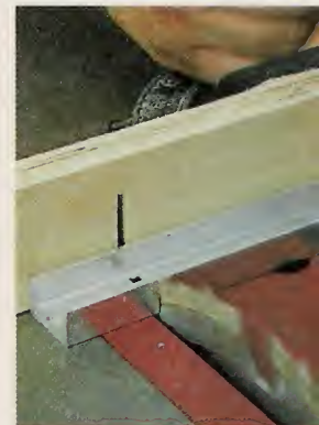
▲ The aluminum channel used for the track and the handle is quite soft, so it cuts easily with a carbide-tipped saw blade.
