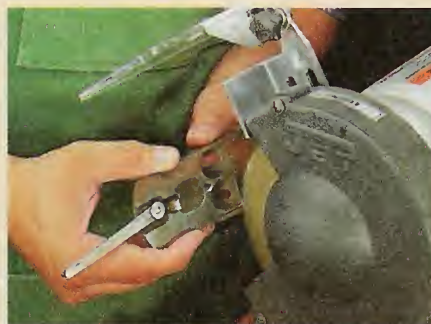
B. Wire Wheel. Using a wire wheel on a grinder makes quick work of removing rust in hard to reach areas.
