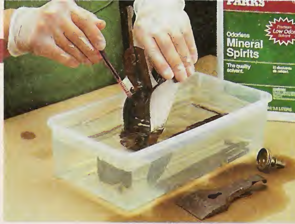
▲ Mineral Spirits Bath. To loosen rust and grime, soak the metal parts of the plane in mineral spirits. Then scrub each part clean with a brush and set it aside to dry.
