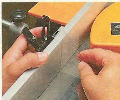
C. Fence. Since there are no stops on the Ryobi fence, a plastic triangle helps square it up to the table.
