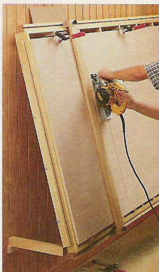
B. Crosscutting. A shorter, vertical fence makes it easy to crosscut sheet goods.
