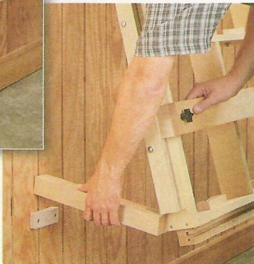
▲ Dual Purpose Legs. To hold the cutting guide at an angle, prop the legs against the wall. With the legs folded down, they support the weight of the cutting guide, see inset photo.
