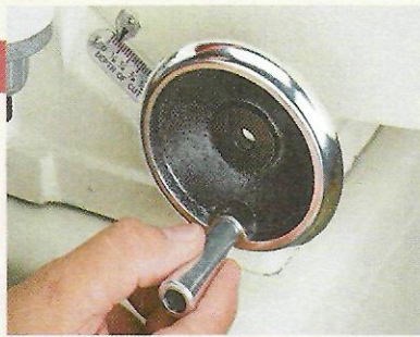
G. Hand Crank. It's easy to make precise depth adjustments with a hand crank on the front of the jointer.
