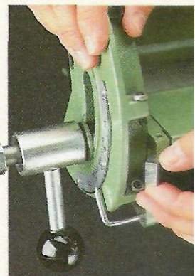
▲ Preset Allen screws contact a flip-out aluminum block to create an accurate stop system.
