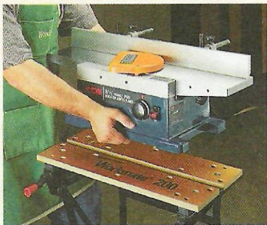
A. Lightweight. A portable jointer is small and lightweight, so it's easy to set up on a temporary worksurface.
