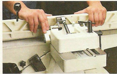
H. Fence. Two machined surfaces and a metal "key" allow this fence to slide smoothly back and forth across the tables.
