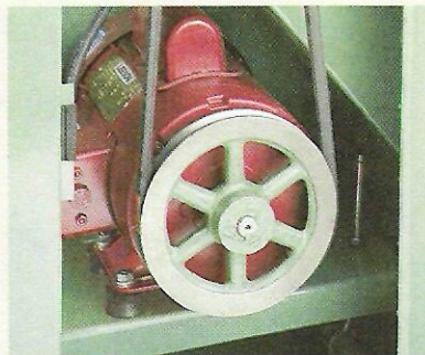
J. Motor. A powerful motor, special mounts, and a balanced pulley make for a smooth-running jointer.
