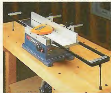
B. Extension Rollers. As an option, you can buy extension rollers to provide support for a long workpiece.
