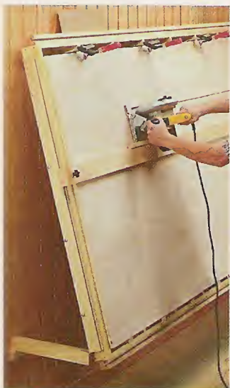
A. Ripping. To get accurate results when ripping, a long, horizontal fence guides the saw.
