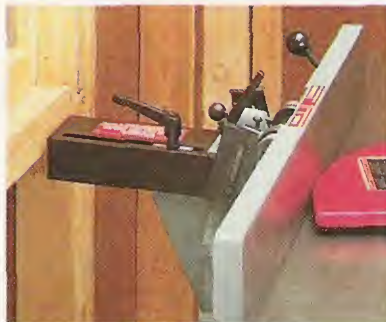
F. Fence. The support on a center-mounted fence sticks out in back, so you can't put the jointer next to a wall.
