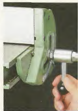
▲ A single lock lever controls the side to side position and the angle of the fence.
