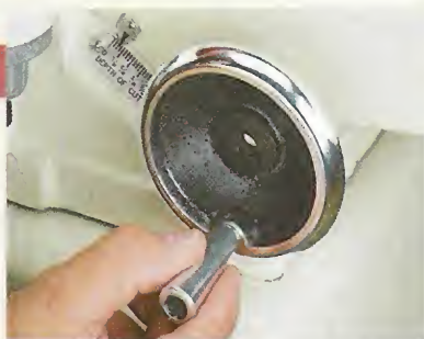
G. Hand Crank. It's easy to make precise depth adjustments with a hand crank on the front of the jointer.
