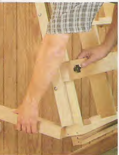
▲ Dual Purpose Legs. To hold the cutting guide at an angle, prop the legs against the wall. With the legs folded down, they support the weight of the cutting guide, see inset photo.
