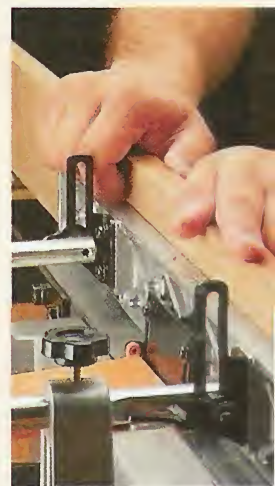
▲ The tall, metal adjustment brackets on this fence are a real knuckle-buster when jointing the edge of a workpiece.
