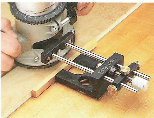
▲ Low-Profile Fence. When the narrow, low-profile fence is mounted to the aluminum body, you can rout a groove (or dado) while the workpiece is clamped flat against a benchtop.
