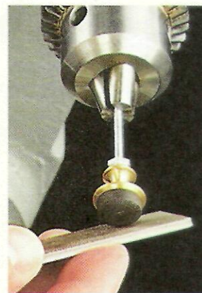
▲ With the knob threaded onto a rod chucked in the drill press, the wood plug is simply filed and sanded to shape. (Two "jam" nuts hold the knob in place.)
