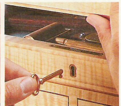
C. Lock System. When closing up shop, slide a brass rod down through the chest (left) to lock the drawers. Then secure the lid with a full-mortise lock and key, see photo at right.
