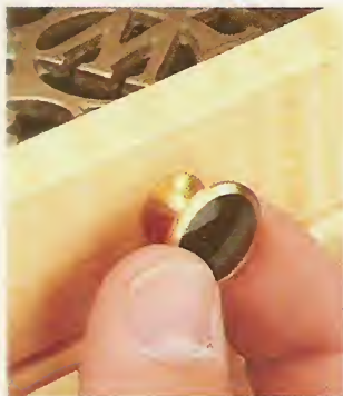
A. Knob. A solid brass knob with an ebony plug highlights the drawers.
