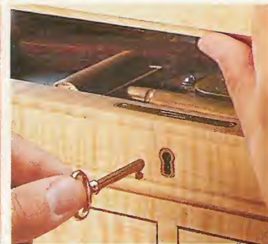
C. Lock System. When closing up shop, slide a brass rod down through the chest (left) to lock the drawers. Then secure the lid with a full-mortise lock and key, see photo at right.
