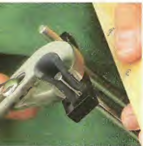
▲ To avoid marring the pins when threading them into the mounting bar, a small piece of rubber is included with the Micro-Fence.
