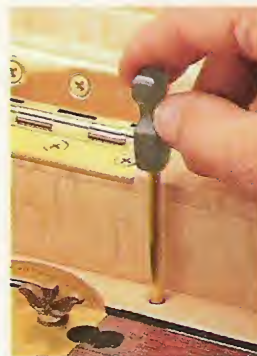
C. Lock System. When closing up shop, slide a brass rod down through the chest (left) to lock the drawers. Then secure the lid with a full-mortise lock and key, see photo at right.
