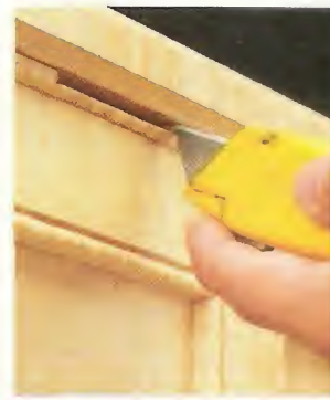
▲ To lay out the location of the hinge on the lid, simply score a line using the mortise in the chest as a guide.
