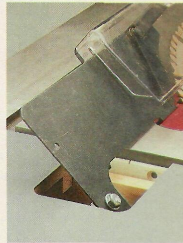
▲ A large opening in the end of the table provides clearance for the blade guard and splitter assembly.
