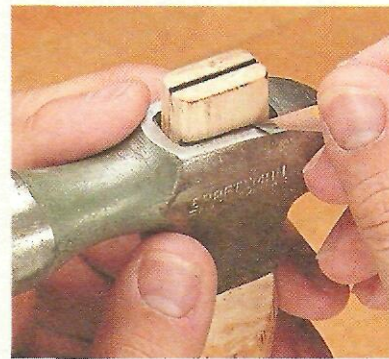
3 With the head "seated" on the shoulder of the tenon, mark the waste at the top end of the handle.
