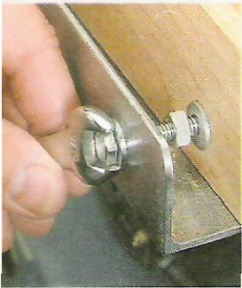
▲ The bolts that hold the rail to the table are also used to adjust it. Here, a quick turn of one of these bolts adjusts the fence for drift.
