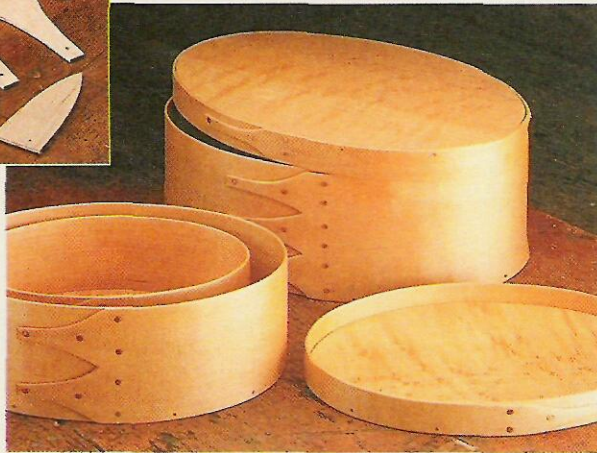
A. Thin Stock. The thin, curved sides of these Shaker boxes are simply resawn from thick stock.
