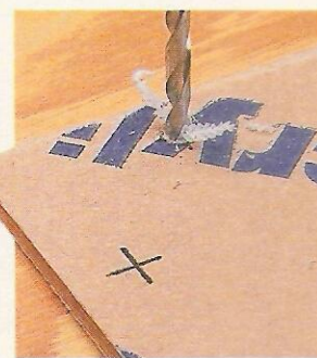
▲ To make it easy to see your layout lines, leave the paper backing on the Plexiglas.
