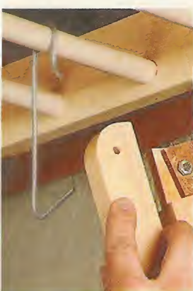
▲ Bending both ends of a stiff wire creates a sturdy hanger that holds jigs on the rack.
