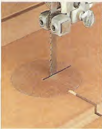
▲ A disk-shaped insert plate covers the throat opening. To prevent it from rotating, a wood "key" fits into the blade slot.
