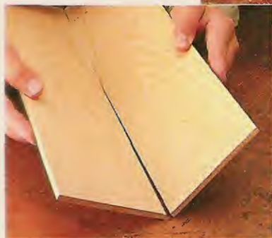
B. Bookmatching. A resawn board can create a dramatic grain pattern with a mirror image on each side.
