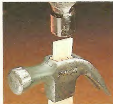
5 Now fit the head back onto the handle, tap in the wood wedge as far as it goes, and trim the waste.
