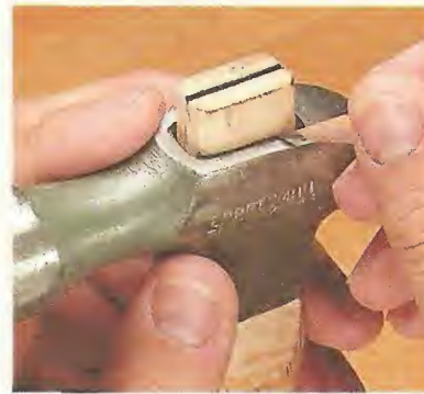
3 With the head "seated" on the shoulder of the tenon, mark the waste at the top end of the handle.
