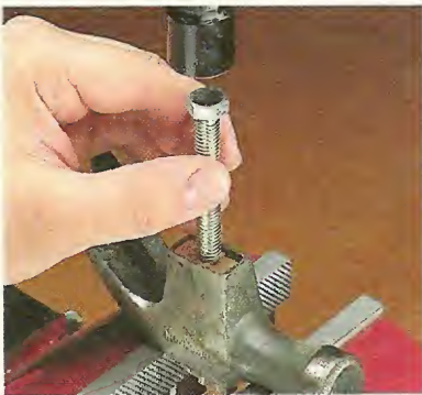
1 To remove the waste in the eye, place the head over an open vise and use a bolt as a punch.
