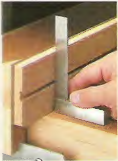
▲ To ensure accurate results, square the table to the blade (upper photo). Then square the fence to the table (lower photo).
