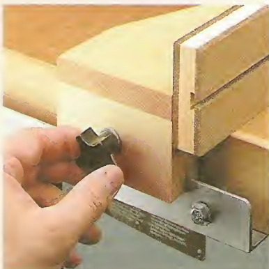
A. Fence Clamp. The band saw fence has a built-in clamp that's locked in place with a plastic knob.
