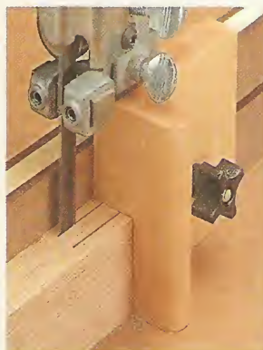
B. Stop/Pivot Block. An adjustable block does double duty as a stop (left) and a pivot block when resawing (right). Tightening a knob clamps the block on the fence.
