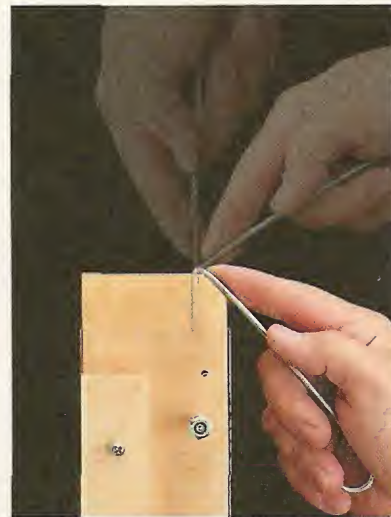
B. Angled Bend. Now fit the straight end of the wire in the hole and bend it around the angled corner of the jig.
