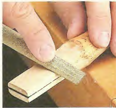
2 A file will help speed up the process of fitting the tenon on the handle into the eye of the head.
