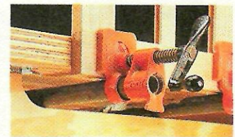
◀ Pipe Clamps. To hold a workpiece against the edge of the bench, slip pipe clamps through the notches at the top of the stretchers.
