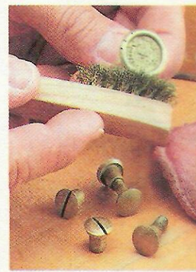
▲ A brass brush and some mineral spirits make quick work of cleaning the hardware that's used to hold the saw blade in the handle.
