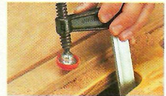
◀ Bar Clamps. Fit the head of a bar clamp down through one of the slots in the top to clamp work near the middle of the benchtop.
