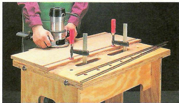
◀ Bar Clamps. Fit the head of a bar clamp down through one of the slots in the top to clamp work near the middle of the benchtop.
