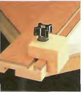
▲ Stop Block. An adjustable stop block provides a quick, accurate way to miter pieces to identical lengths.
