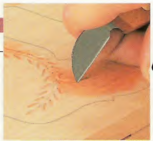
▲ Stem. When carving the curved stems of the wheat pattern, the idea is to make two slicing cuts to remove a thin ribbon of wood.
