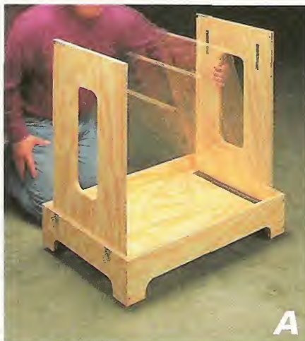
Turn a single sheet of plywood and a few pieces of hardware into a portable workbench that “knocks down” for compact storage.
