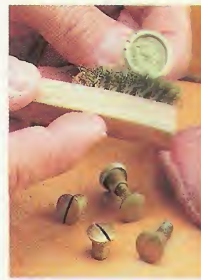
▲ A brass brush and some mineral spirits make quick work of cleaning the hardware that's used to hold the saw blade in the handle.
