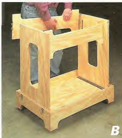
Turn a single sheet of plywood and a few pieces of hardware into a portable workbench that “knocks down” for compact storage.
