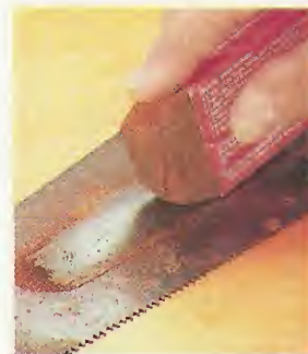
▲ A rubber block embedded with silicon carbide "erases" the rust on the saw blade.
