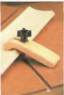
▲ Hold-Down. For safety, this simple hold-down clamps work securely against the base of the jig.
