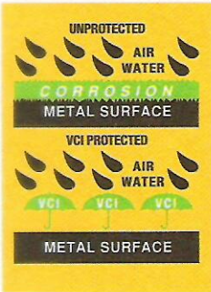
▲ Bullfrog products emit microscopic VCIs to create a protective umbrella on metal surfaces.
