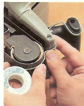
▲ To "copy" the irregular shape on the end of the sander, wrap a short length of solder around the housing.
