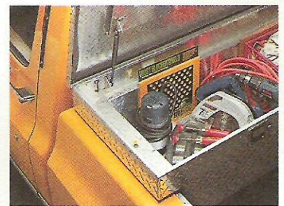
C. Shield. A perforated shield seals metal surfaces in large areas (up to 100 cubic feet) as in this toolbox.
