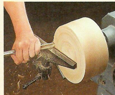
6 Finally, reposition the toolrest and flatten the face of the blank before you begin shaping the bowl.
