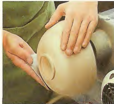
3 To smooth the surface, sand the spinning bowl by hand using progressively finer grits (80 to 320-grit).
