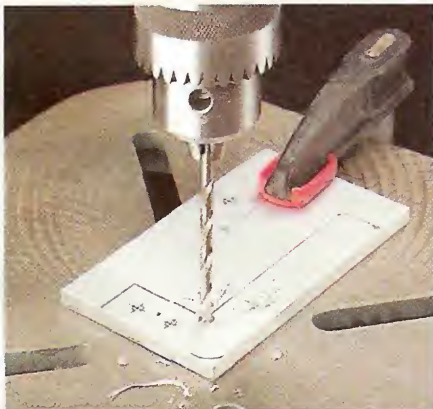
1 Drill Holes. After laying out both stops on the aluminum plate, clamp it securely to the drill press table. Then use a twist bit to drill the holes.
