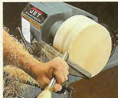
5 After mounting the blank, set the lathe to run at a slow speed (600 RPM) and "true up" the outside.
