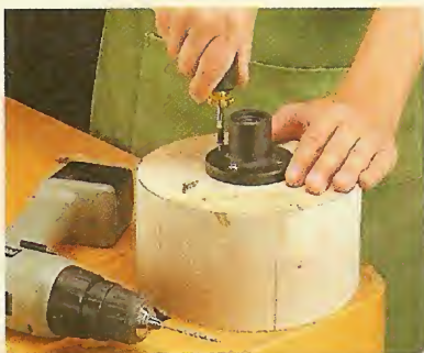
4 Once the waste is removed, center the faceplate on the blank and then screw it in place.
