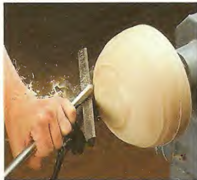
1 Using smooth, sweeping cuts, work from the base of the bowl to the rim to turn it to shape.
