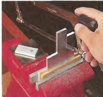
2 Cut to Shape. A hack saw slices easily through the aluminum when cutting the extension stop (lying on the vise) and the L-shaped stop to shape.
