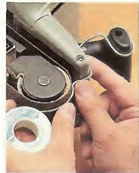
▲ To "copy" the irregular shape on the end of the sander, wrap a short length of solder around the housing.
