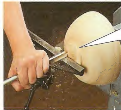
2 Now cut a recess in the base with a bowl gouge (detail 'a') and square it up with a scraper (detail 'b').
