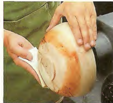
4 With the lathe off, apply a coat of finish and let it soak in. Then turn the lathe on and buff the finish.
