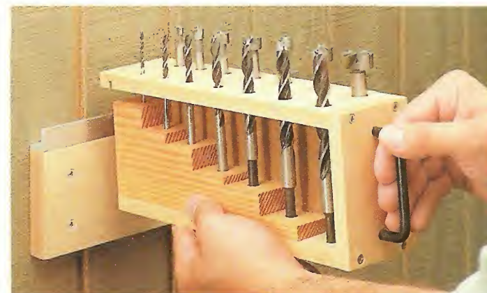
▲ Removable Hangers. Each hanger hooks onto a metal rail attached to a wall-mounted cleat. To drill a hole in a project at the bench (or around the house), simply lift the hanger off the rail and take the bits with you.
