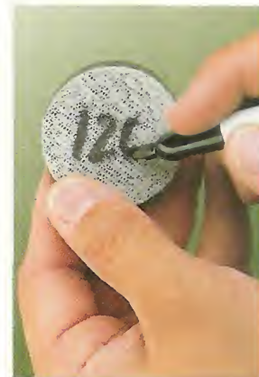
▲ The grit sizes on the sanding disks are hard to see. So to avoid using the wrong disk, I write the grit size on the back with a permanent marker.
