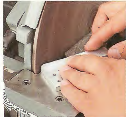
3 Sand the Corners. To create a gentle radius on the corners, sand them smooth with a disk sander. Or if you prefer, use a file and sanding block.
