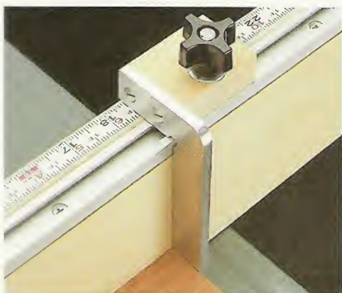
A. Stop Block. By sliding this stop block to the desired mark on a measuring tape, it's quick and easy to cut boards accurately to length.
