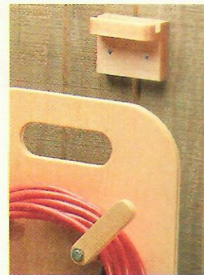
▲ To hold a single caddy, an L-shaped wood block with a groove in the top provides a handy, wall-mounted hanger.
