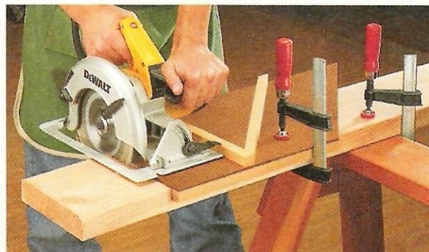
▲ 90° Crosscuts. Simply turn the guide around and align the opposite end to make a 90° crosscut. To square the jig, make sure the cleat is tight against the workpiece.
