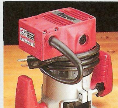
B. Cord Wrap . To reduce the strain on a power cord, make a large loop before wrapping it around the tool.
