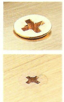
▲ To create an almost invisible seam, drill the countersinks so the screw heads sit "proud" (upper photo). Then file and sand them flush (lower photo).
