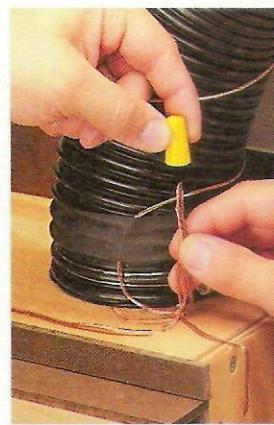
▲ To complete the grounding path, "tie" the ends of the wires together with wire nuts.
