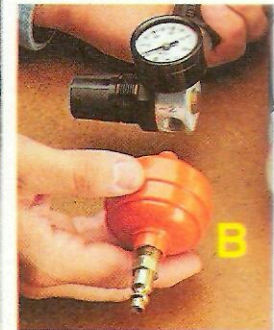
▲ Conversion Gun. With a conversion gun, air is supplied by a compressor. To avoid contaminating the finish, it's important to remove moisture from the air by installing a permanent trap (A) or disposable filter (B).
