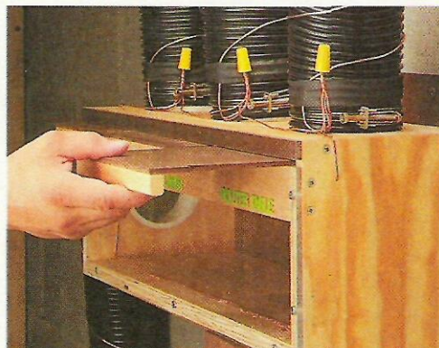
B. Dust Control Box. To direct dust and chips from the tool you're using to the dust collector, simply slide open the blast gate for that tool.
