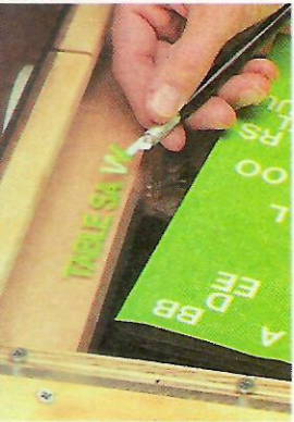
▲ To see which blast gate controls the air flow at each tool, I labeled the front of the box with self-adhesive letters.
