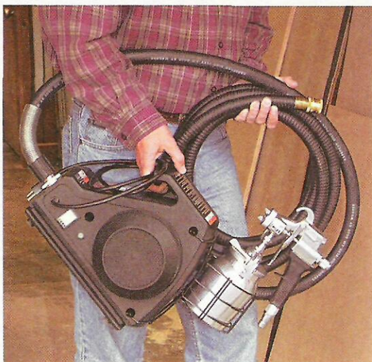
▲ Turbine. A turbine-style HVLP system is a lightweight, portable unit that produces clean, dry air to atomize the finish from the spray gun.
