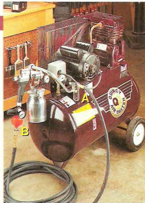
▲ Conversion Gun. With a conversion gun, air is supplied by a compressor. To avoid contaminating the finish, it's important to remove moisture from the air by installing a permanent trap (A) or disposable filter (B).
