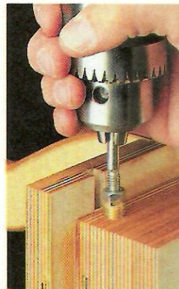
▲ To prevent an insert from going in crooked, tighten a cutoff bolt with a "jam" nut in the drill press and turn the chuck by hand.
