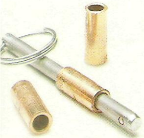
▲ Indexing System Hardware. A cotterless hitch pin that fits into bronze bushings forms a precise indexing system.
