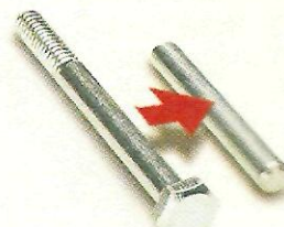
▲ Steel Pins. The pivot pin and the stop are cut from the unthreaded portion of a bolt.
