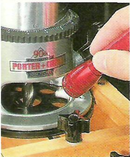
▲ Shining a small flashlight down through the router and platform makes it easy to align the router bit with the layout lines for the mortise.
