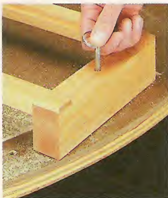
▲ Index Pin. A metal pin locks the saw carriage in place for precise cuts every time.
