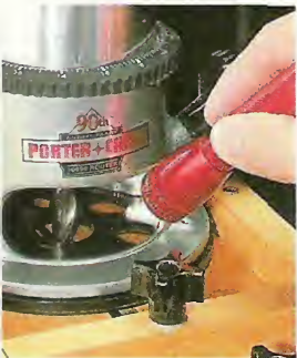
▲ Shining a small flashlight down through the router and platform makes it easy to align the router bit with the layout lines for the mortise.
