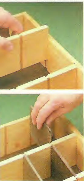
▲ Adjustable dividers allow the compartments in the insert to be rearranged as your storage needs change.
