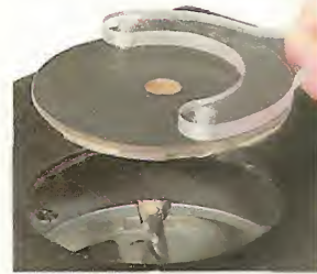
▲ Insert Ring. A spanner wrench is included with the Rout-R-Lift to remove the phenolic ring.
