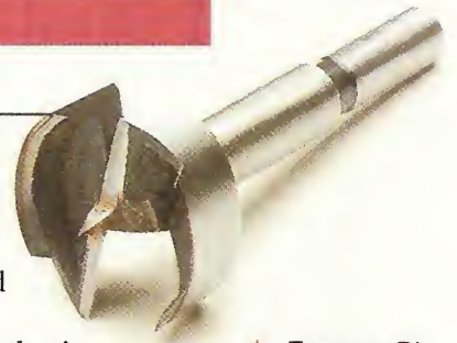
▲ Forstner Bit. This bit is great for drilling flat-bottomed holes.
