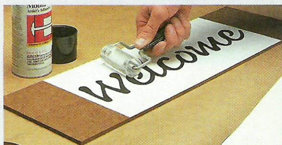
▲ Create Pattern. After making a photocopy of the pattern, use a spray adhesive to temporarily attach the pattern to an oversize hardboard template.
