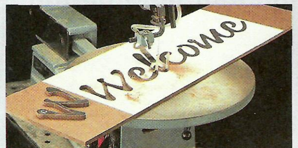
▲ Cut Out Template. Using a scroll saw (or jig saw), remove the waste from the template. Then smooth the inside edges of the template with sandpaper.
