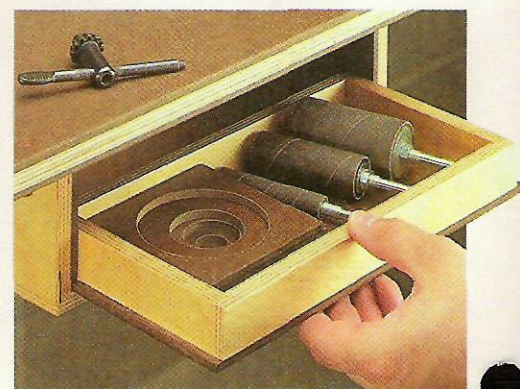
Storage Tray. A small, pull-out tray provides a convenient place for storing a chuck key, drill bits, or sanding drums.
