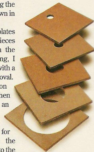
▲ Hardboard Inserts. You can customize the sizes of the openings in the inserts to match your sanding drums.
