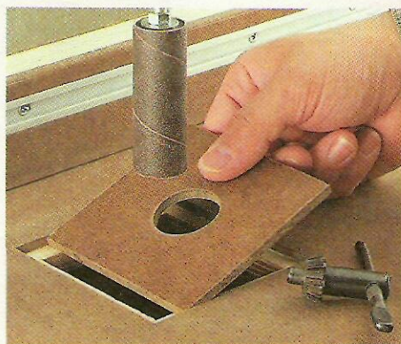
Sanding Drum Inserts. Replaceable inserts can be interchanged quickly for various diameters of sanding drums.
