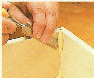
4 Remove Excess. Finally, remove the dried "foam" by scraping (shown above left) or sanding. Removing glue from hard-to-reach areas like a corner (photo at right) is a snap with a sharp chisel — it "pops" right off.
