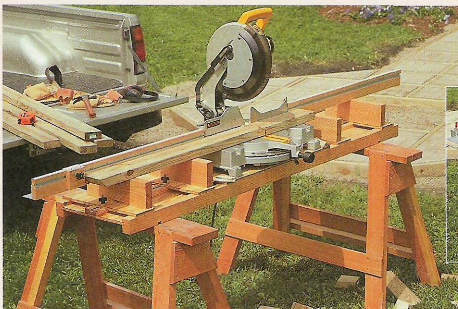
▲ Portable. A lightweight design and carrying handles make the miter saw station easy to move to the job site.
