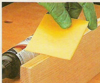
2 Spread. Use a flexible piece of plastic or laminate to spread the glue evenly along the edge.
