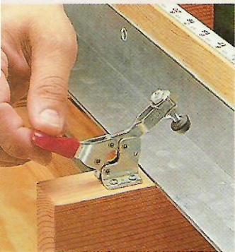
▲ Small toggle clamps make it easy to quickly adjust the position of the supports and fences.
