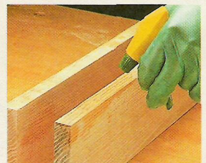
3 Mist. To provide the moisture to cure the glue, lightly mist the edge of the mating workpiece.
