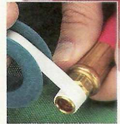
▲ Air-Tight Seal. To get a good seal between couplers, wrap the threaded ends of the fittings with Teflon tape.
