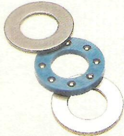
▲ Bearing. A pair of washers and a thrust bearing make it easy to turn the handwheel to adjust the height.
