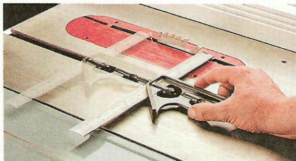
▲ Check Blade. First place the square in the miter slot and set it to touch a tooth. Rotate the blade and slide the square back to touch the same tooth. If it's not parallel, the trunnion will need to be adjusted.
