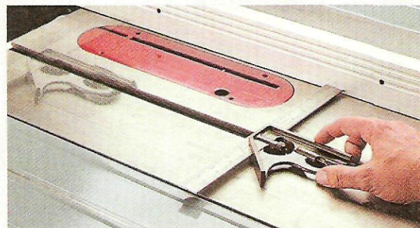
▲ Check Rip Fence. Once the blade is aligned, adjust the square out, as shown. Then slide the rip fence in until they touch. Now lock the fence down and move the square back to see if it's parallel to the miter gauge slot.
