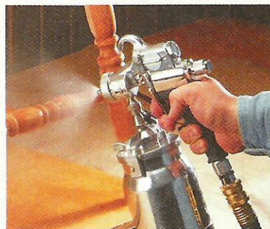
▲ Spray Finishing. Larger compressors will handle a spray gun for applying a perfect finish.
