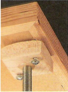
▲ Support Blocks. The key to allowing the top to move freely is to "loosely" screw the support blocks to the top.
