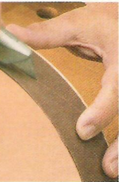
▲ Scarf Joint. Use a utility knife to cut a scarf joint in the sandpaper. Then glue the sandpaper to the wheel with contact adhesive. (See page 35 for sandpaper sources.)
