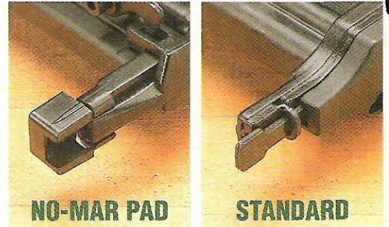
▲ Safety. A nose-mounted safety prevents the nailer from firing inadvertently. And a pad (left) on some nailers prevents the nose from denting the workpiece as it recoils, unlike a standard nose (right).
