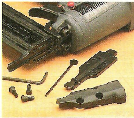
▲ Jam Clearing. Brad nailers that require you to disassemble the nose with an Allen wrench (left) can be a big hassle when you need to clear a jam. But clearing a jam is an easy task on a brad nailer with a quick-release latch (right).
