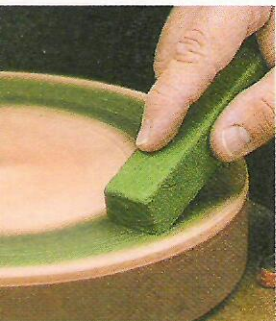
▲ Honing Compound. Before honing the edge of your tool on the wheel, charge the leather with honing compound.
