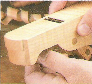
▲ Adjustable Throat. To accommodate the thickness of the shaving, the throat opening can be adjusted easily.
