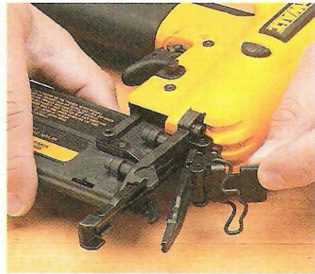
▲ Jam Clearing. Brad nailers that require you to disassemble the nose with an Allen wrench (left) can be a big hassle when you need to clear a jam. But clearing a jam is an easy task on a brad nailer with a quick-release latch (right).
