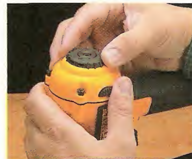
▲ Exhaust. Redirecting the air (and oil) from you and your workpiece is easy with an adjustable exhaust port.
