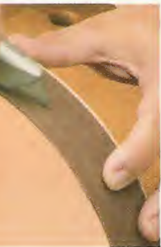
▲ Scarf Joint. Use a utility knife to cut a scarf joint in the sandpaper. Then glue the sandpaper to the wheel with contact adhesive. (See page 35 for sandpaper sources.)
