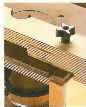
▲ Fence. This adjustable fence slides in the T-slots on the router base plate.
