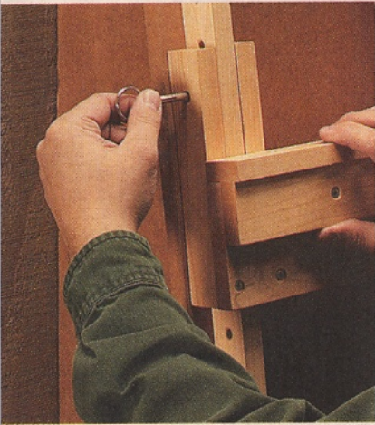
▲ Clamp Bar Adjustment. A simple quick-release pin holds the clamp bar in position once it's been adjusted to match the size of the panel being glued up.
