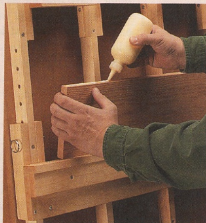
▲ Add Glue. After adjusting the lower clamp bar, apply glue to each workpiece and stack to form panel.
