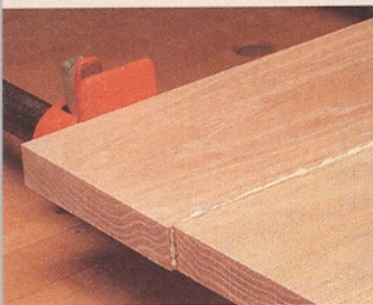
▲ Clamping. A thin bead of glue indicates good pressure along the joint line.
