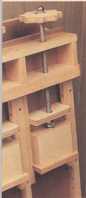
▲ Clamp Heads. Individual clamp heads are used to apply pressure evenly across the top edge of the panel.
