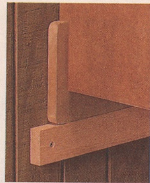
▲ Cleat Support. A temporary cleat makes it easy to keep the clamping station level when you attach it to the wall.
