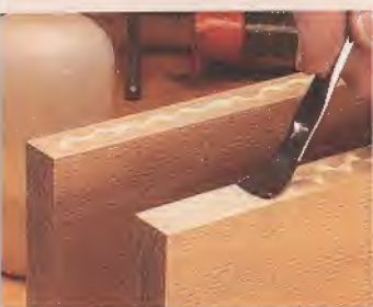
▲ Gluing. A bristle brush is a quick and easy way to spread a smooth, even layer of glue along the edge of a board.
