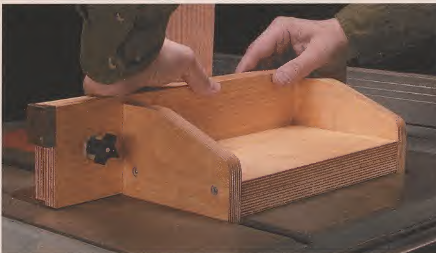
▲ Two are Better Than One. The sides of this jig form runners that ride in the miter gauge slots of your table saw.
