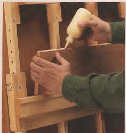
▲ Add Glue. After adjusting the lower clamp bar, apply glue to each workpiece and stack to form panel.
