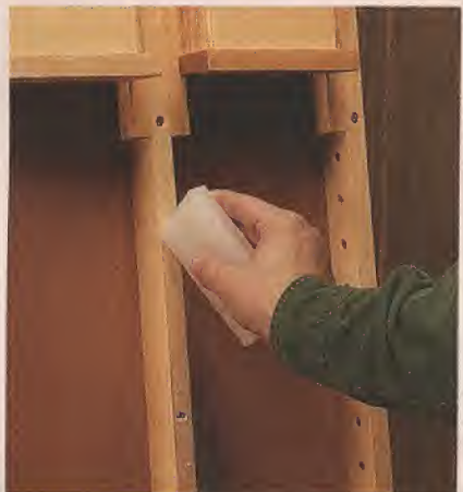
▲ Apply Wax. To prevent glue (and the panel) from sticking to the station, rub paraffin wax on the vertical rails.
