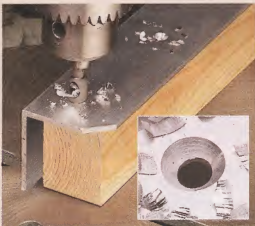
▲ Metal Work. Smooth countersinks in soft metal, like brass or the aluminum shown above, are a snap with a Weldon countersink.
