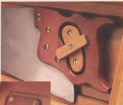
▲ Saw Storage. Mounted to the inside of the lid, a custom-fitted wood block and turn-button secures the saw handle. And a leather "pocket" holds the end of the saw blade.
