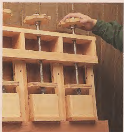
▲ Clamp. With the workpieces in place, apply pressure evenly across the panel by tightening each clamp head.
