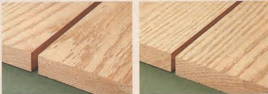
▲ Appearance. To get a good-looking, wide panel, it's best to avoid drawing attention to a joint line. To do this, arrange boards so curved patterns merge (left) and straight-grained boards are positioned to create an "invisible" joint (right).
