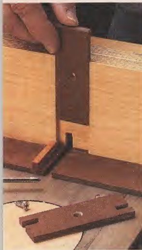
▲ Replaceable Insert. A hardboard backing insert can be easily replaced as it gets chewed up through use.
