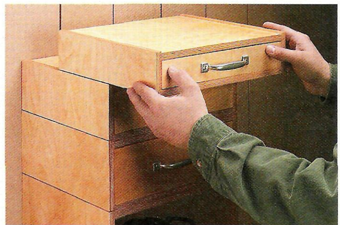
Stack 'Em Up. These drawer units stack on top of one another to create a complete router storage system. The top of each unit is recessed to hold the unit above.
