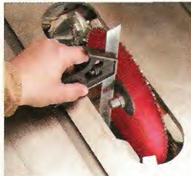
▲ Square the Blade. Using a combination square, check that the saw blade is square to the table.
