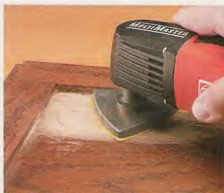
▲ The MultiMaster 's smooth operation makes it easy to sand into tight places like the corner of this frame and panel door.
