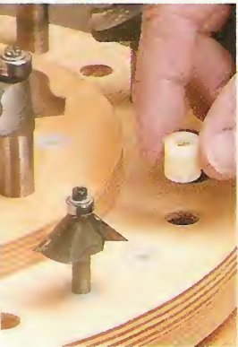
Nylon Bushing. In order to accommodate 1/4" shank router bits, a nylon bushing can be used to reduce the size of the hole.
