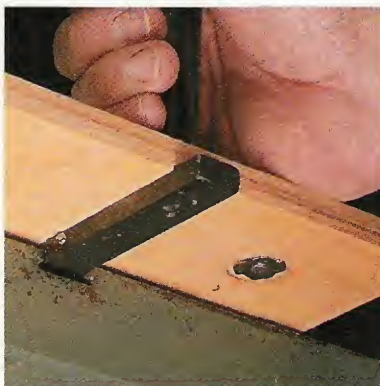
Miter Bar. Adjustable ball bearings keep this miter bar (and the sled) running firm and true in the miter slot.
