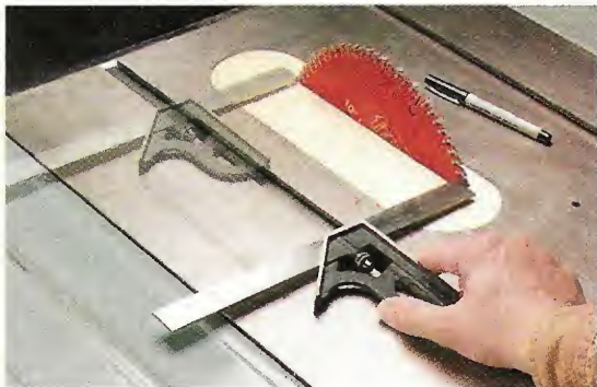
▲ Alignment. Verify that the saw blade is parallel to the miter slot by checking the position of a single tooth at both the front and rear of the table saw.
