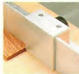
▲ Stop Block. For thin materials, the stop block can be reversed, allowing you to butt the workpiece against the clamping plate.
