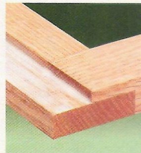
▲ Cleaner Glue-ups. You'll have less glue squeeze out on the inside of the cabinet if you only spread the glue to the corner of the rabbet.
