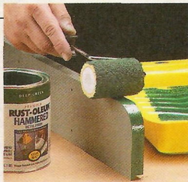
Step 1. After priming the workpiece, roll the paint onto the edges first, using a short-nap roller.
