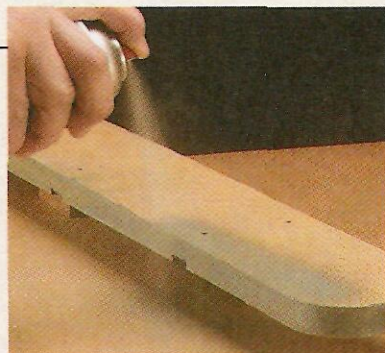
Step 2. Because the faces don't absorb the primer as much as the edges, a single coat is fine here.
